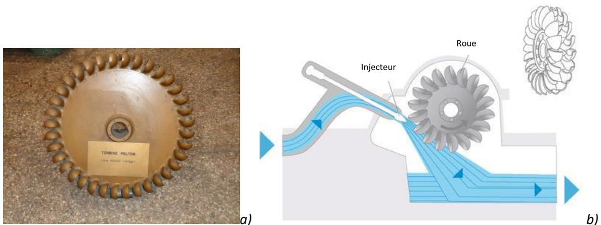
**Figure 1.** a) Pelton-type turbine (photo P. Sagnes – OFB) ; b) operating principle (www.landeskraftwerke.bayern).
