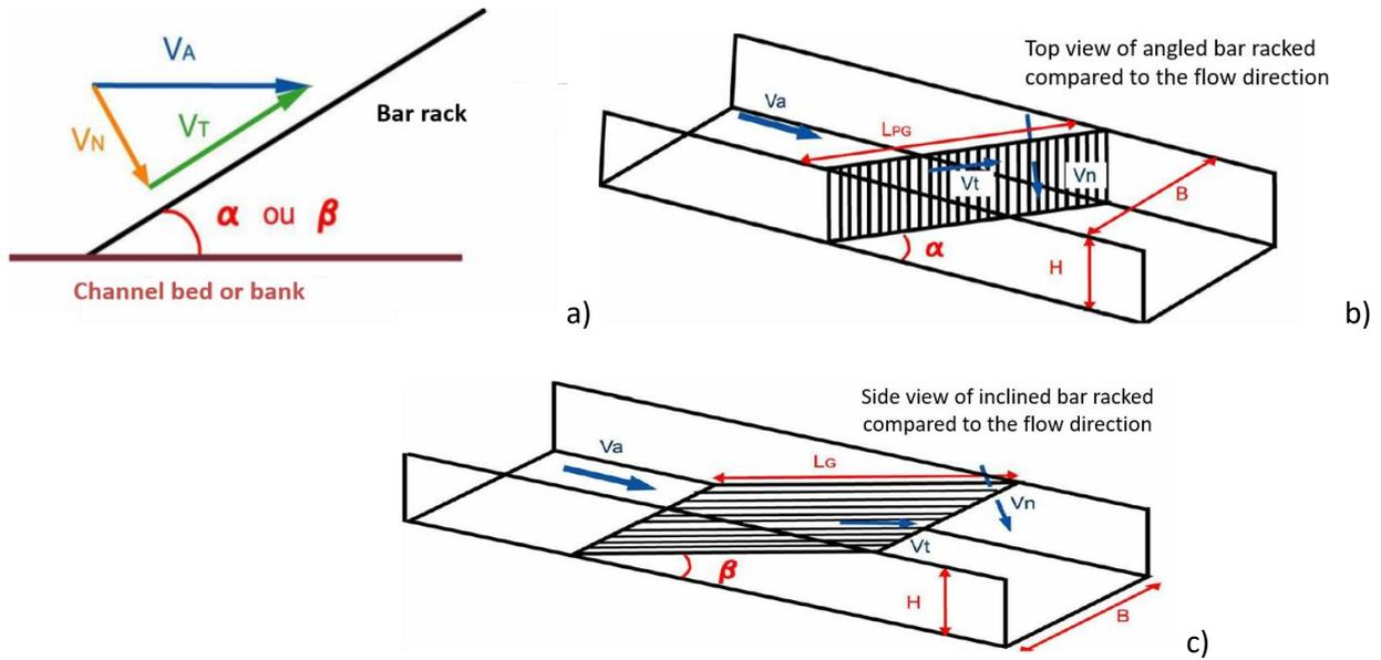
**Figure 22.** a) Components of the outflow speed approaching a bar rack (cf. Figure 13) and angle to the bank [ $\alpha$ , angled bar rack, b)] incline to the bottom of the channel [ $\beta$ , inclined bar rack, c)]. According to Courret & Larinier (2008).
