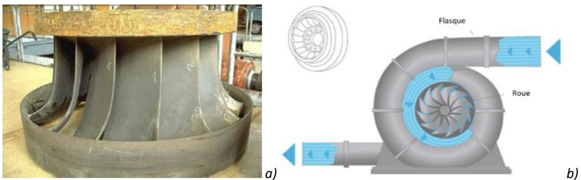
**Figure 2.** a) Francis-type turbine (photo P. Sagnes – OFB); b) operating principle ([www.landeskraftwerke.bayern](http://www.landeskraftwerke.bayern)).
