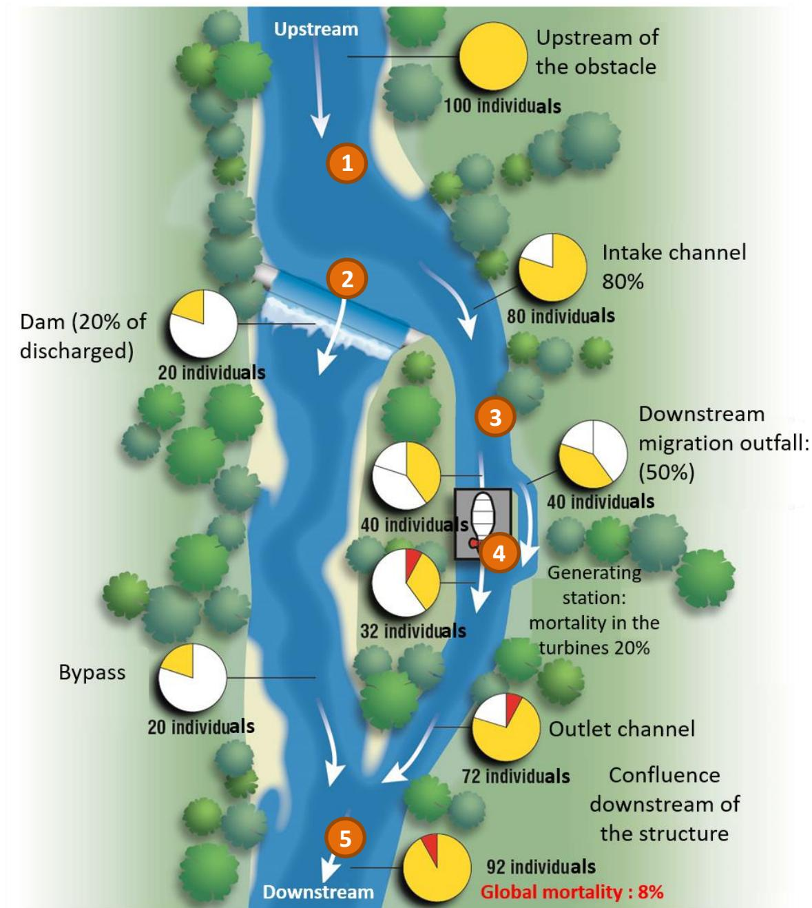
**Figure 9.** Five stages in order to estimate a mortality rate for downstream migrating eels at the level of a hydropower facility. In yellow: proportion of live individuals; in red: proportion of dead individuals According to Baudoin et al. (2014).
