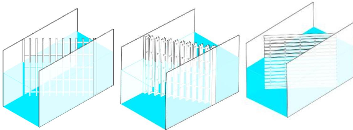
**Figure 23.** Schematic diagram of the 3 bar assembly methods in the case of angled racks: "conventional" rack on the left, bars aligned in the direction of the outflow in the centre, and horizontal bars on the right (according to Lemkecher et al., accepted).
