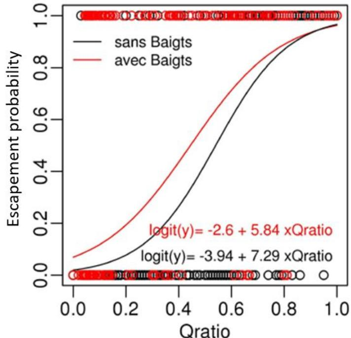
**Figure 16.** Predicting the escapement probability of eels migrating downstream through the spillway of a dam according to the distribution of the flow between the dam and the hydropower generating station ( $Qratio = \text{overflow discharge at the dam divided by the total flow of the watercourse}$ ). The black curve is the general formula (see text). According to Bau et al. (2013).
