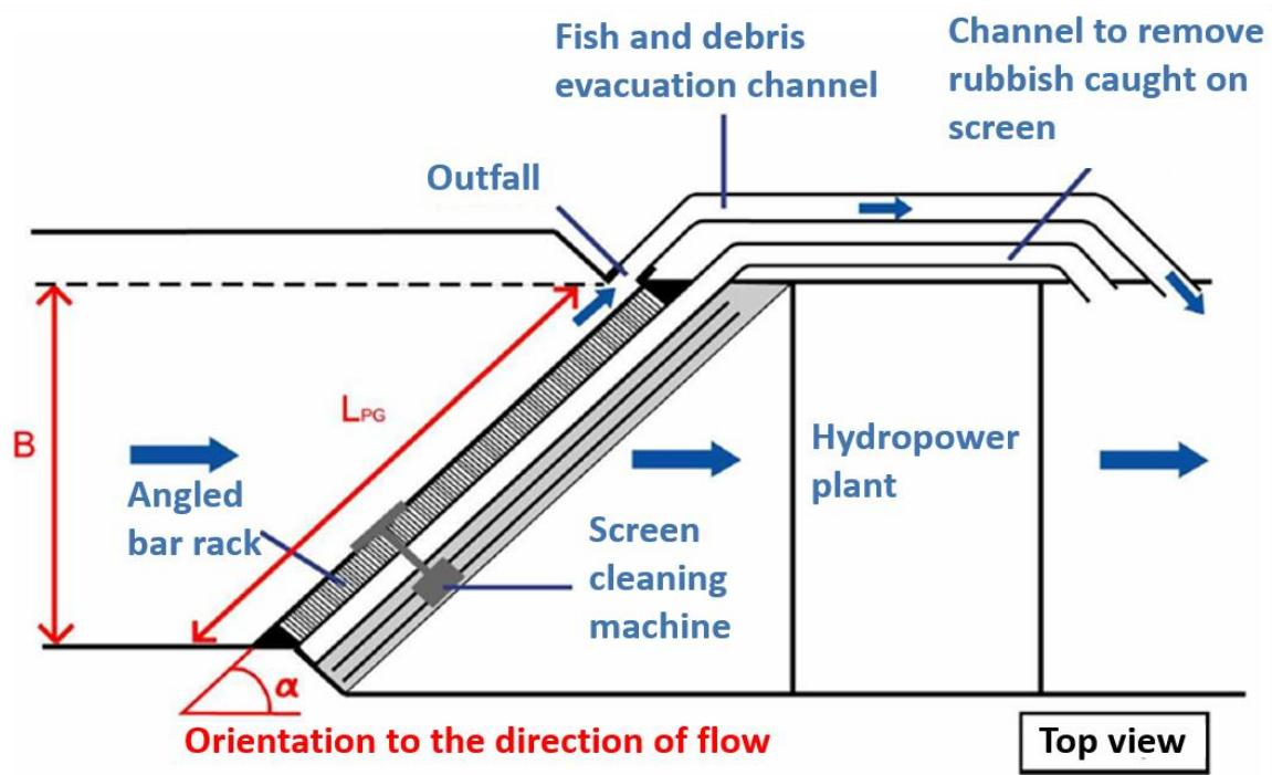
**Figure 7.** Angled bar rack, top view. According to Courret & Larinier (2008).
