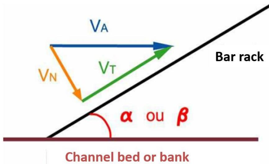
**Figure 13.** The different components of the outflow speed upstream of an inclined bar rack.  $V_A$ : approach speed;  $V_N$ : normal speed;  $V_T$ : tangential speed. According to Courret & Larinier (2008).
