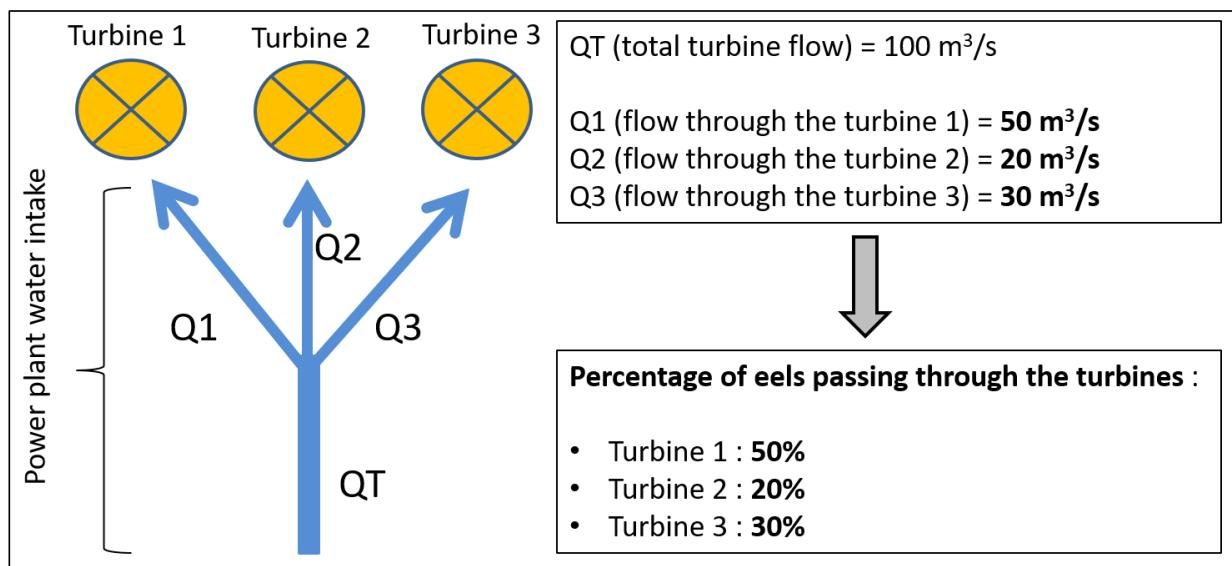
**Figure 28.** Distribution of flows between three turbines supplied by a single water intake and deduction of the share of eels passing through each of them
