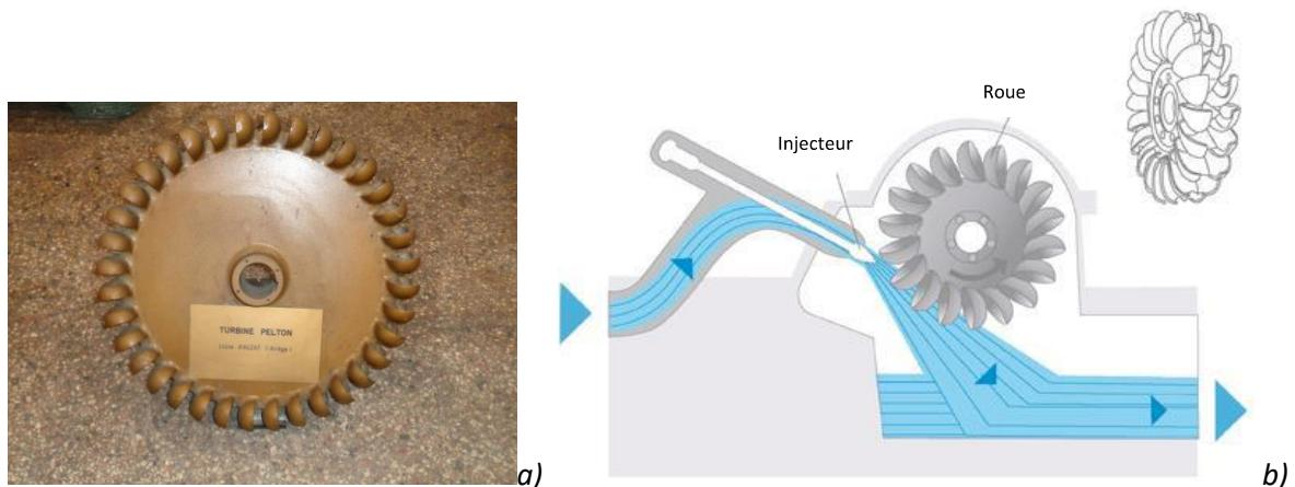
**Figure 1.** a) Pelton-type turbine (photo P. Sagnes – OFB) ; b) operating principle ([www.landeskraftwerke.bayern](http://www.landeskraftwerke.bayern)).
