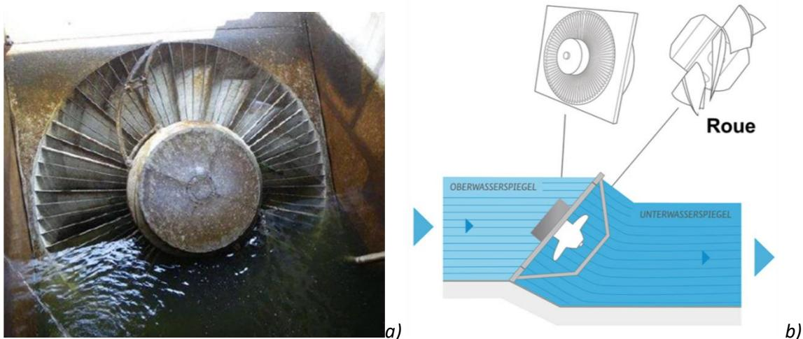
**Figure 4.** a) Ichtyophile© VLH turbine (photo ECOGEA); b) operating principle ([www.landeskraftwerke.bayern](http://www.landeskraftwerke.bayern)).
