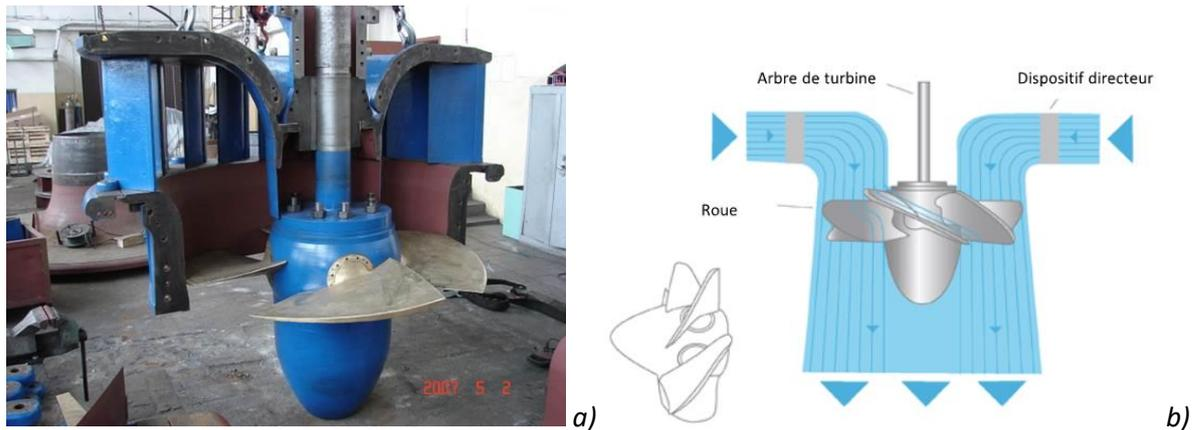
**Figure 3.** a) Kaplan-type turbine (photo D.Courret – OFB); b) operating principle (www.landeskraftwerke.bayern).
