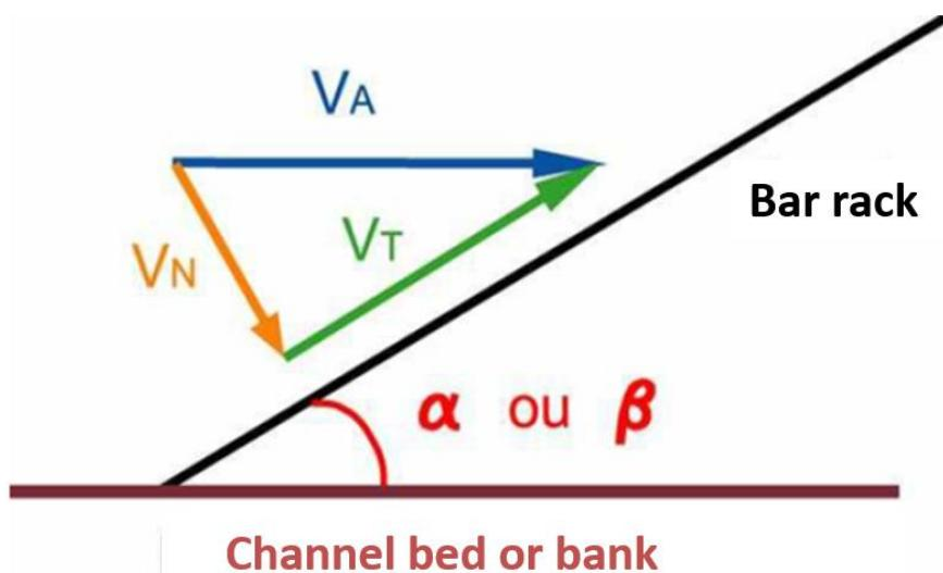
**Figure 13.** The different components of the outflow speed upstream of an inclined bar rack.
