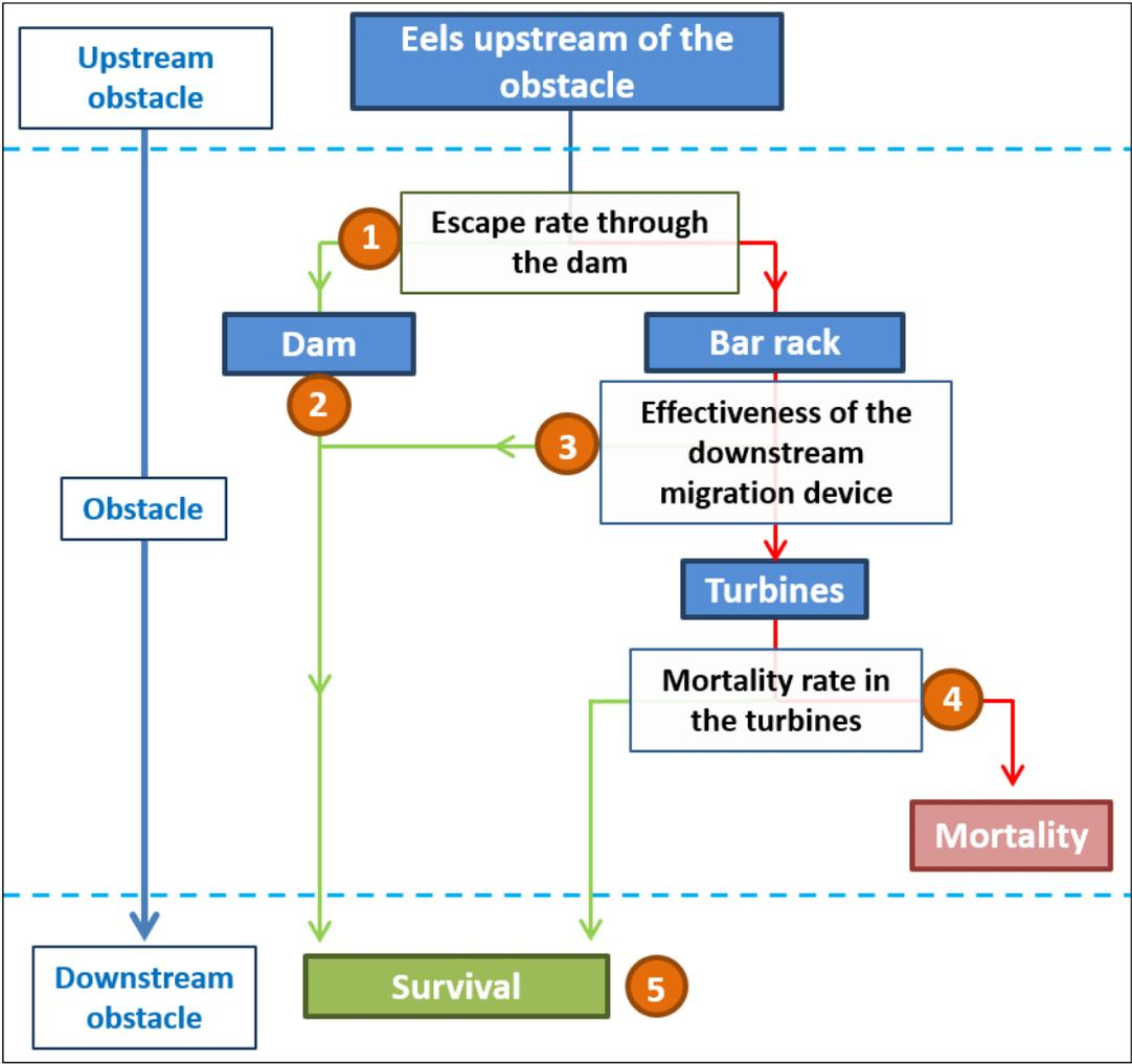
**Figure 29.** Different stages allowing the overall mortality rate of fishing migrating downstream at a hydropower facility.
