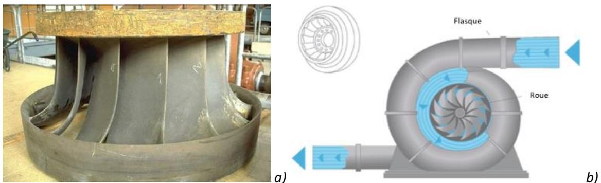
**Figure 2.** a) Francis-type turbine (photo P. Sagnes – OFB); b) operating principle ([www.landeskraftwerke.bayern](http://www.landeskraftwerke.bayern)).
