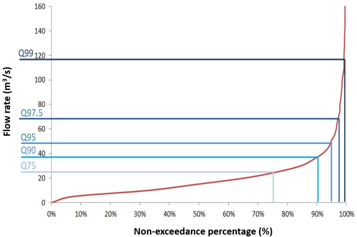
**Figure 11.** Example of a classified flow curve (Gave d'Aspe, France, between 2000 and 2011) during the eel downstream migration period (from October to January here), which allows the characteristics flows of a watercourse for a given period to be defined ( $Q_x$  = non-exceeded flow  $x\%$  to the time). Curve established during the data analysis of SUDOANG deliverable 2.2.2.
