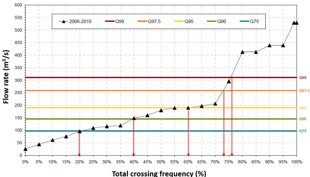
**Figure 14.** Characteristic flows of the eel downstream migration periods on the Gave de Pau (between 2006 and 2010) and combined passages of the individuals. Qx = flow not exceeded during x% of time. According to Bau *et al.* (2013).
