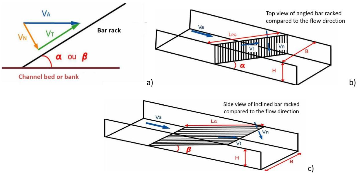
**Figure 22.** a) Components of the outflow speed approaching a bar rack (cf. Figure 13) and angle to the bank [ $\alpha$ , angled bar rack, b)] incline to the bottom of the channel [ $\beta$ , inclined bar rack, c)]. According to Courret & Larinier (2008).
