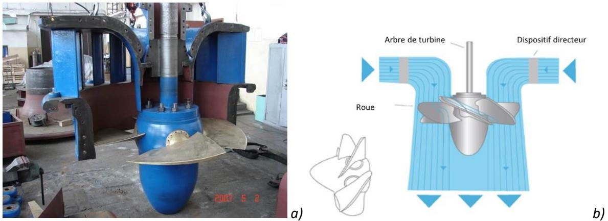
**Figure 3.** a) Kaplan-type turbine (photo D.Courret – OFB); b) operating principle ([www.landeskraftwerke.bayern](http://www.landeskraftwerke.bayern)).
