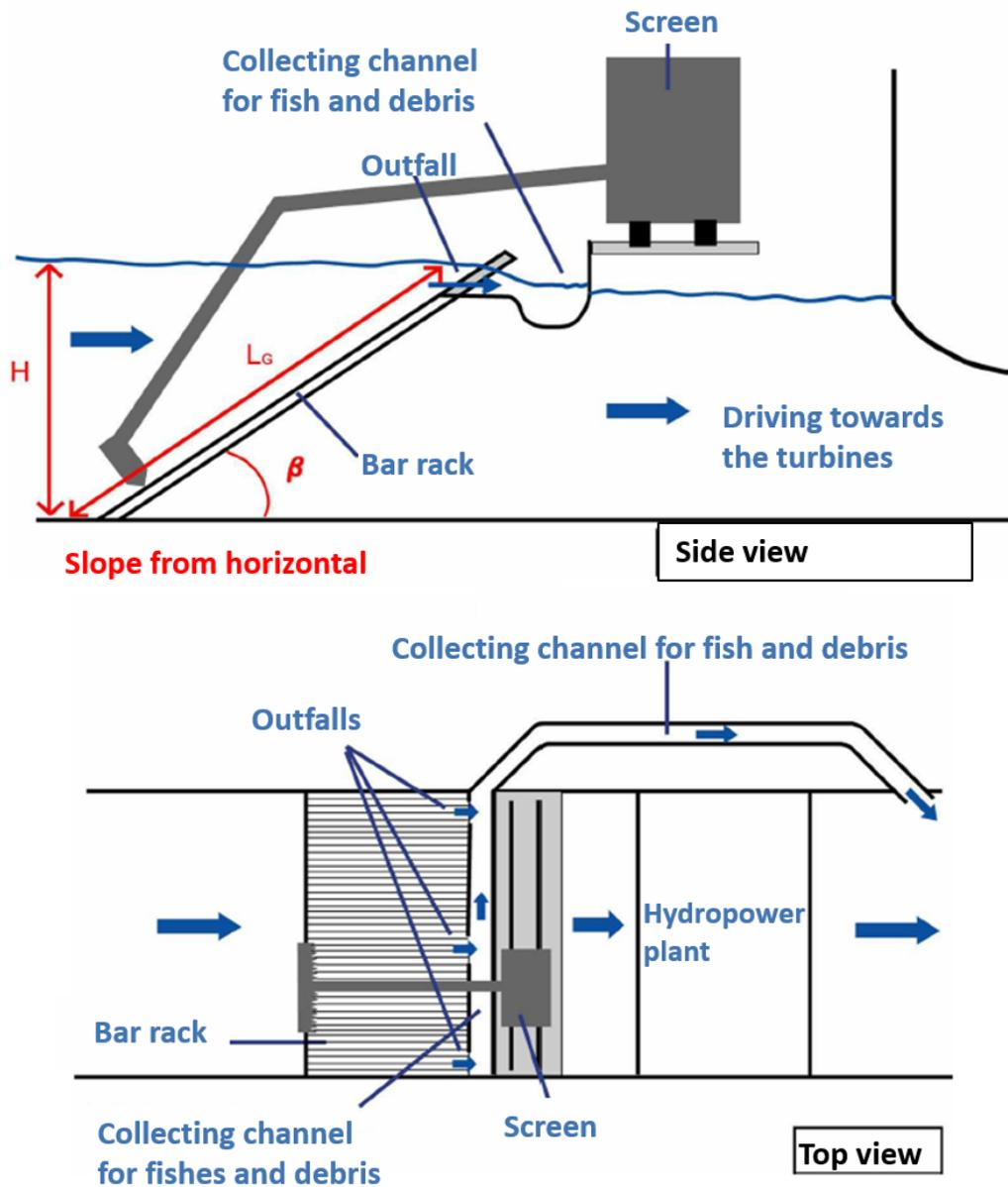
**Figure 8.** Inclined bar rack. Top: side view; bottom: top view. According to Courret & Larinier (2008).
