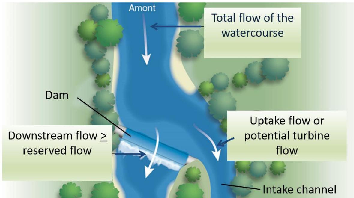
**Figure 12.** Diagram of the distribution of the flows at the level of a weir. According to Baudoin et al. (2014).
